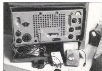
Fig. 3: The Mark 123 'Spy' set. The unit comprises the receiver on the left, transmitter on the right with the p.s.u. in the centre. The box on the lower right is the 'tape measure' housing for the wire antenna.
