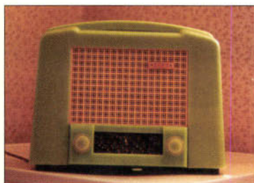
Fig. 5: The fully restored (green Bakelite cabinet) Ecko U122 receiver. One of the rarest 'vintage' sets is the famous 'Green Onyx' Ecko Bakelite cabinet type 'Saucepan' shaped receivers of which only two or three were ever made.
