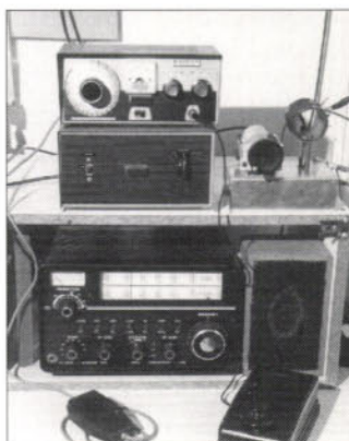
Fig. 1: The Codar AT5 transmitter and Drake 2B receiver, with a G4BXD a.t.u. and Type D RAF Morse key.
