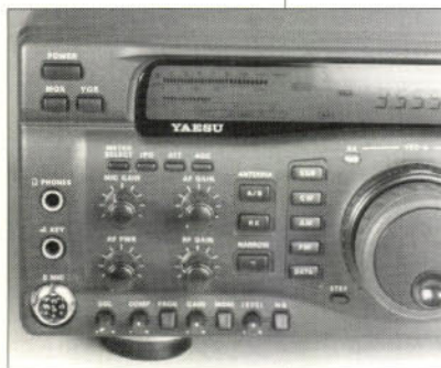
The left-hand side of the FT-920's front panel. The outer 'collar' control mounted directly behind the main tuning knob operates the 'Shuttle Jog' tuning control (see text).
