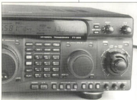
The right-hand side of the FT-920's front panel. The main tuning knob is just visible to the left, with the VFO-B knob almost central. (This also provides auxiliary tuning - see text for comments). The DSP controls are on the far right with the 'hour and minute hand' type rotary controls providing adjustment for 'Low Cut' DSP filtering and 'High cut' filtering (see text).
