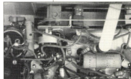
Fig. 2: The underside of a (in surprisingly good condition) Ecko U122 receiver showing waxed paper capacitors before replacement (see text).
